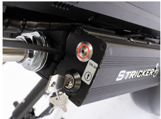
Fig. 18: The reverse light on the control lights up when reverse gear is activated
