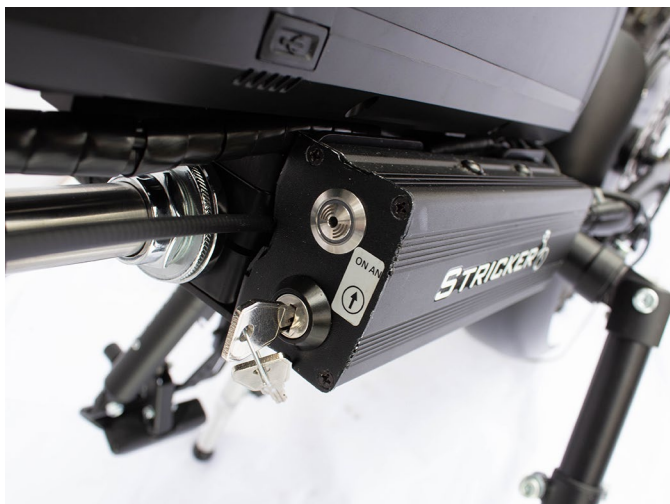
Fig. 11: Key switch on battery and control
