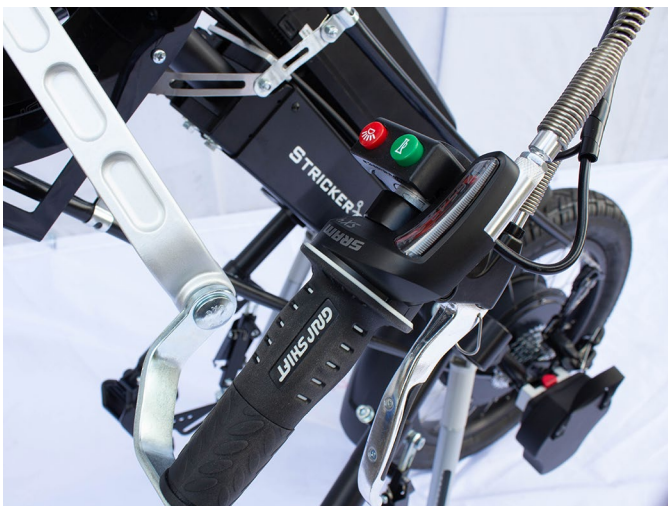
Fig. 19: Brake lever with brake contact and initiation of recuperation (interrupter contact is only connected to the right brake lever.)
