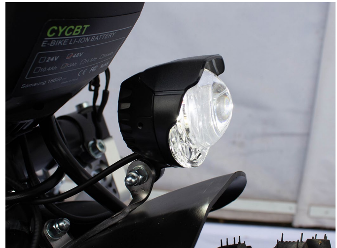
Fig. 17: Adjustment of the inclination of the lamp with integrated horn
